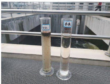
Comparison of sewage before and after treatment in the sewage treatment plant
